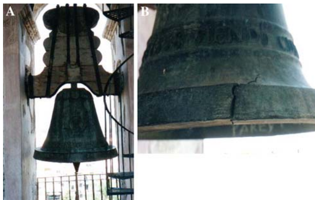
Fig. 2 a Bell in first floor, north side. b Fracture of west bell in second floor
